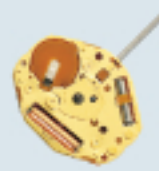
GL30 GILT height 2.28mm 3 year battery life (SR6215W)
