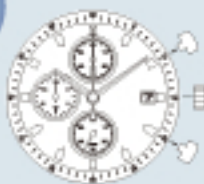
OS10 height 4.13mm date chrono hour/min/sec 3 year battery life (SR927W)
