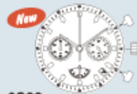
OS22 height 5.10mm date chrono min/sec, 24 hour FAST TURNING CHRONO HAND: 1/20 sec. measuring indicated by 6H second hand (operative in specific models) 2 year battery life (SR927W)
